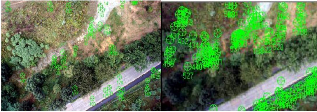
Figure 5: Images showing the distribution of tie points in an image as a result of variation in parameters as shown in table 3
